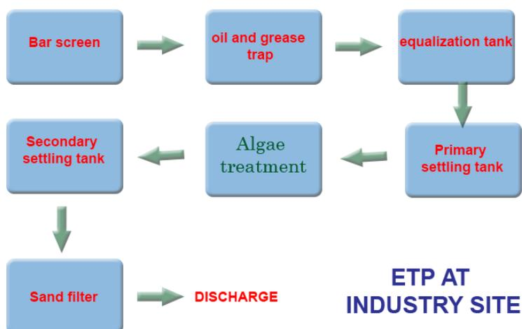
Fig 2. Shows the ETP at leather industry site in Kanpur
