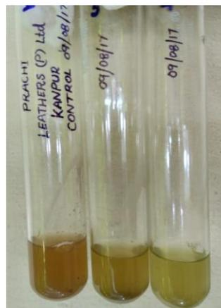
Fig 4 Showing growth of micro algae and reduction in colour of the raw effluent from leather industry
