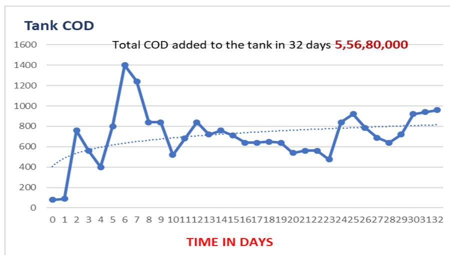
Fig. 5. The trend of COD of leather industry effluent over a period of 32 days in a semi-continuous addition of raw effluent into the treatment tank.
