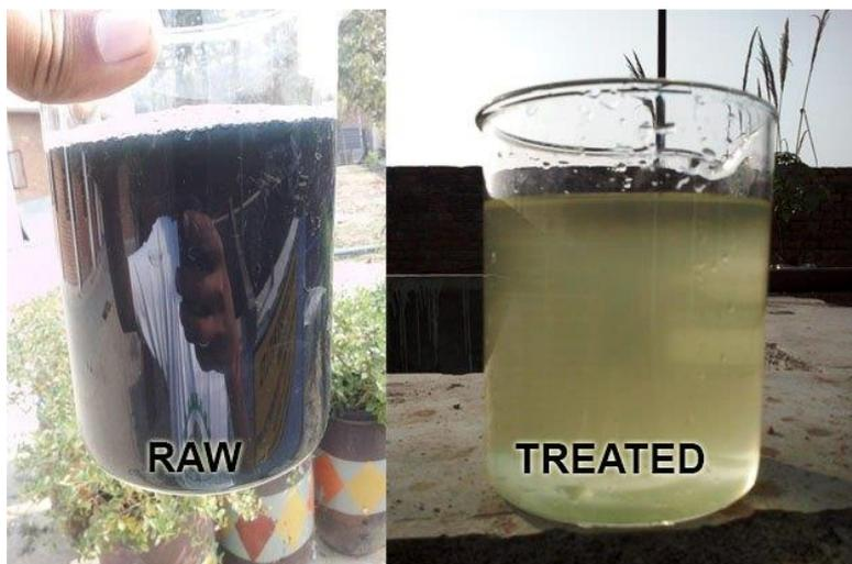
Fig 6 Showing colour removal by micro algae treatment in leather industry effluent
