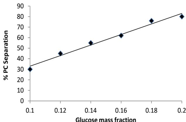
**Figure 5 Separation of phycocyanin from *Spirulina plantesis* using sugaring out (Temperature 4°C, ACN: buffer ratio 1)**
